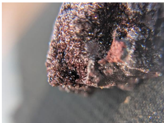
Fig 5.3.13.13: Cuprite in quartz vein under the lens near Burera
