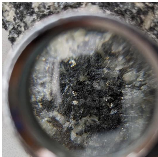
Fig 5.3.8.8: Pyrite (Under hand Lens) in Diorite near Sirsee
