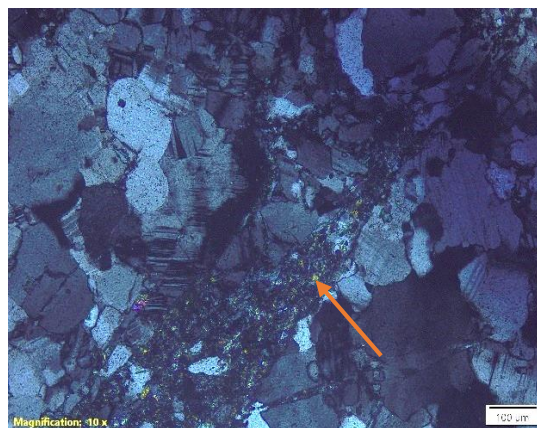
Fig 5.3.4.2: Medium-grained granite with quartz (undulose extinction), altered feldspar and epidote (orange arrow), under cross polar.
