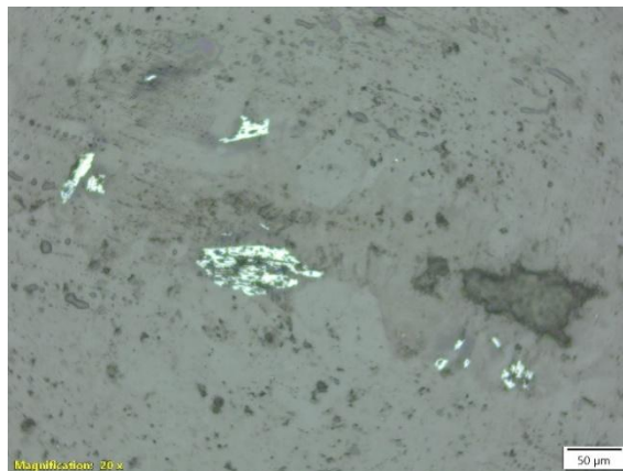
Fig 5.3.13.8: Fine grained to medium grained quartz in quartz vein with pyrite or chalcopyrite, under reflected light.
