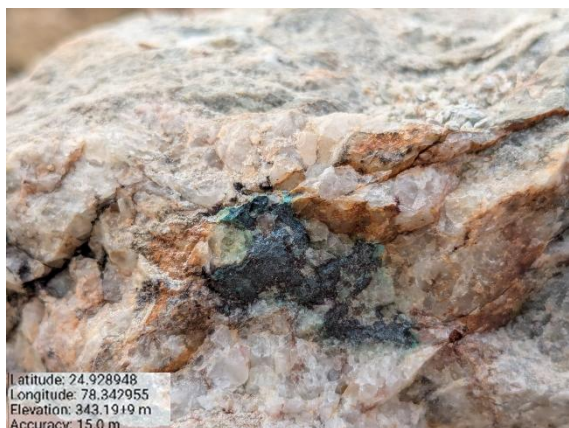
Fig 5.3.13.11: Molybdenite and Malachite associated with quartz, near Burera.
