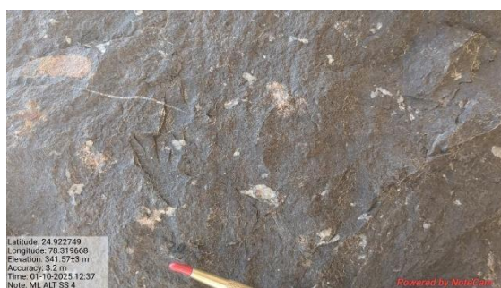
Fig 5.3.11.1: Basalt with quartz blebs, near Burera Village.
