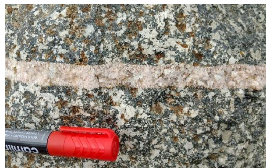
Fig 5.3.5.2: The medium to coarse-grained equigranular granite veins in diorite, near Sirsee.
