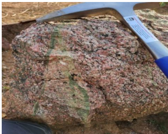
Fig 5.3.4.1: Medium-grained equigranular granite with epidote veins (yellow arrow), south of Mailar mine.
