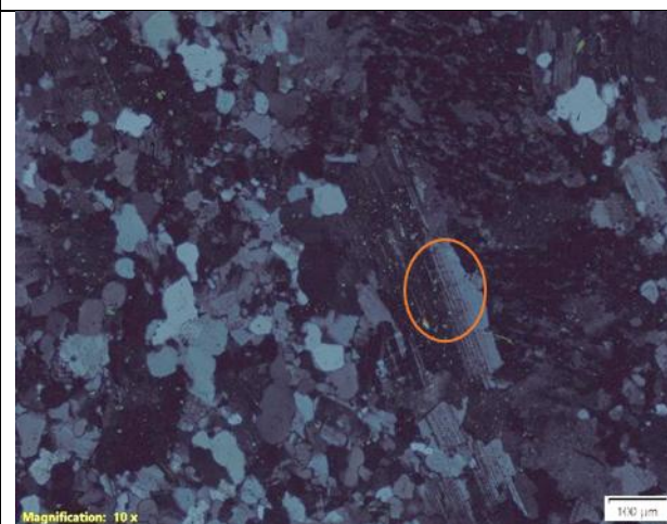
Fig 5.3.1.5 Plagioclase phenocrysts with epidote inclusions showing signatures of propylitic alteration, under cross polar.
