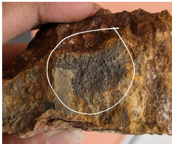
Fig 5.3.7.2: Presence of pyrite and chalcopyrite with other sulphides
