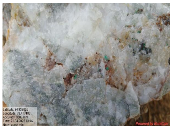
Fig 5.3.13.16: Malachite and Silver within Quartz vein, near Lalaon
