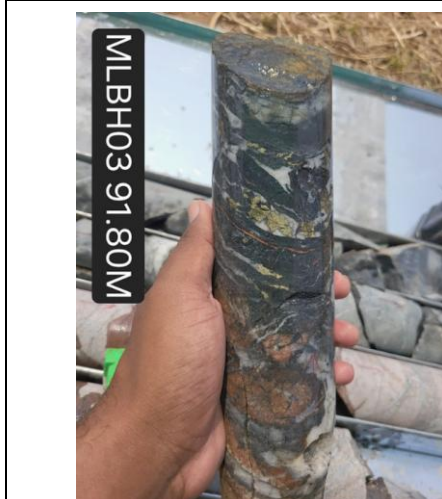
Fig 11.5.2.8: The presence of chalcopyrite within the Drill Core Sample (one meter composite sample gives 3% Copper).
