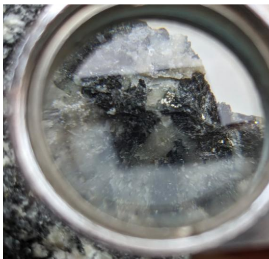
Fig 5.3.8.7: Chalcopyrite (Under hand Lens) in Diorite near Sirsee
